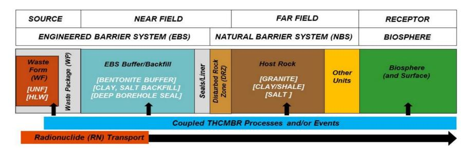
Schematic diagram of the conceptual model framework of a generic geologic disposal system
