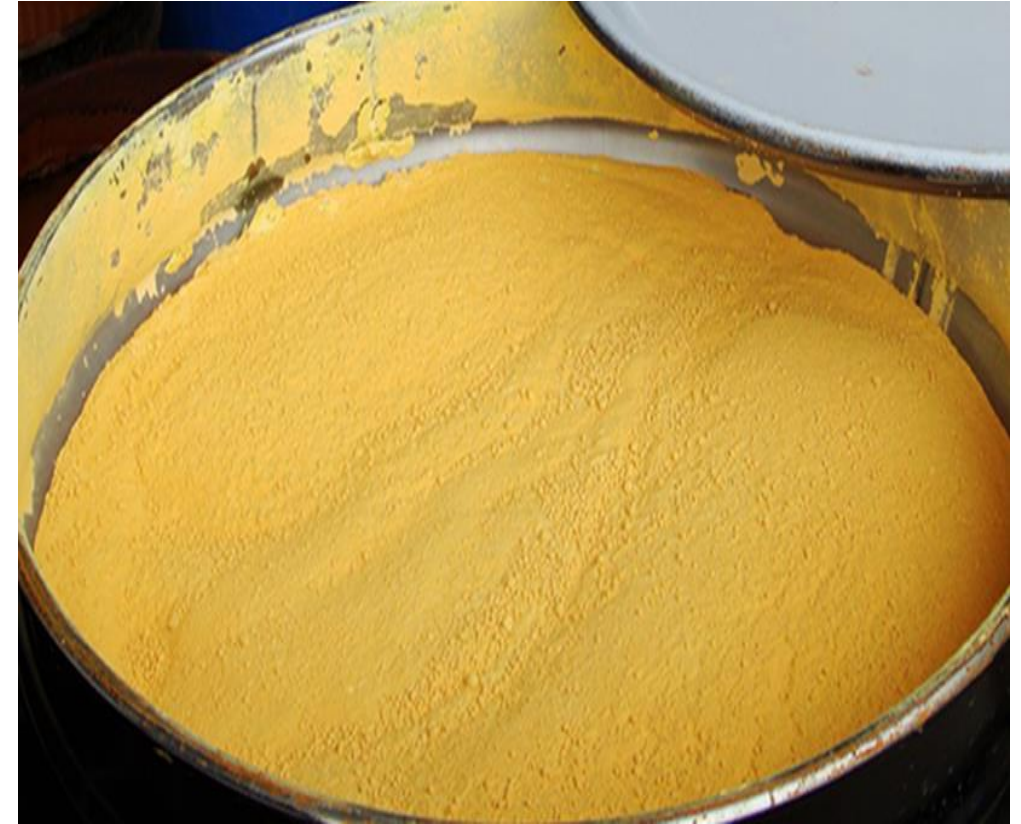
Uranium oxide "yellowcake" is processed from uranium ore before enrichment.
