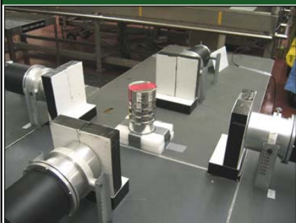
Four large liquid-scintillator detectors are shown here being used to analyze a storage can of MOX fuel pins.
