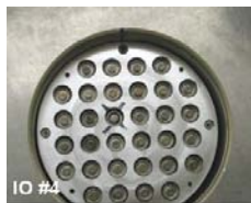
Assembly of Fuel Elements with Single Defect (marked by “x”)
