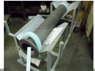
SiC test section – 600 graphite spheres - 1.25 kw/sphere (max)
