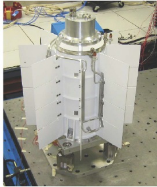
Multi-Mission Radioisotope Thermoelectric Generator (MMRTG) for NASA
