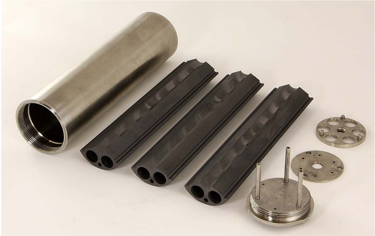
Figure 9. Components of the FS-1 in-core capsule. Left-to-right are the outer nickel capsule, the three sections of the graphite sample and flibe holder, and, top-to-bottom on the right, the bottom graphite support/spacer, the top cover plate, and the capsule lid. The combination of the bottom spacer, top cover plate, and the pins protruding from the bottom of the lid ensure that under in-core, nuclear heating conditions, the flibe melts from the top down. The pins protruding from the bottom of the lid also ensure that the graphite rotates when the lid is screwed onto the capsule bottom. Two of these pins are hollow and will have Inconel sheathed, type-K thermocouples brazed into them. The bottom plate has a threaded hole in its center so the graphite pieces can be pulled from the nickel capsule after irradiation.
