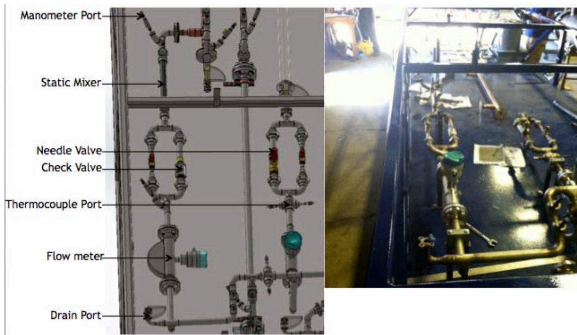
Figure 10. CAD model and current fabrication status of bottom of CIET primary loop (photograph taken on 9/27/2013).
