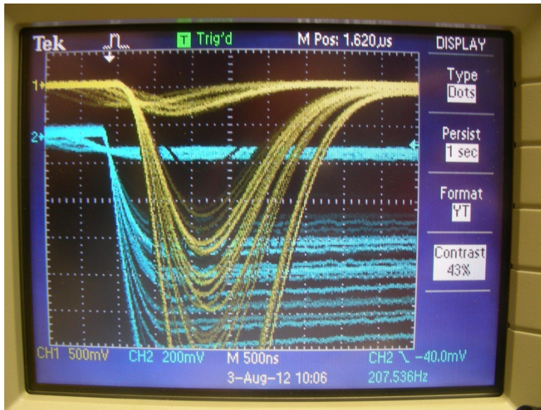
Fig. 45. Photograph of oscilloscope traces showing the preamplifier output (blue) and shaper output (yellow).
