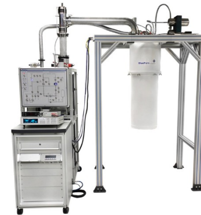
Microcalorimeter gamma spectrometer, Los Alamos National Laboratory and University of Colorado Boulder
