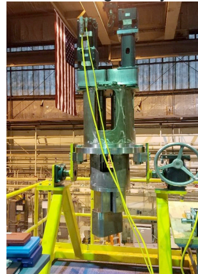
METL Test Article – Gear Test Assembly (example)
