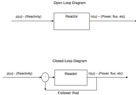
Figure 1: Open Loop and Closed Loop Schematic
