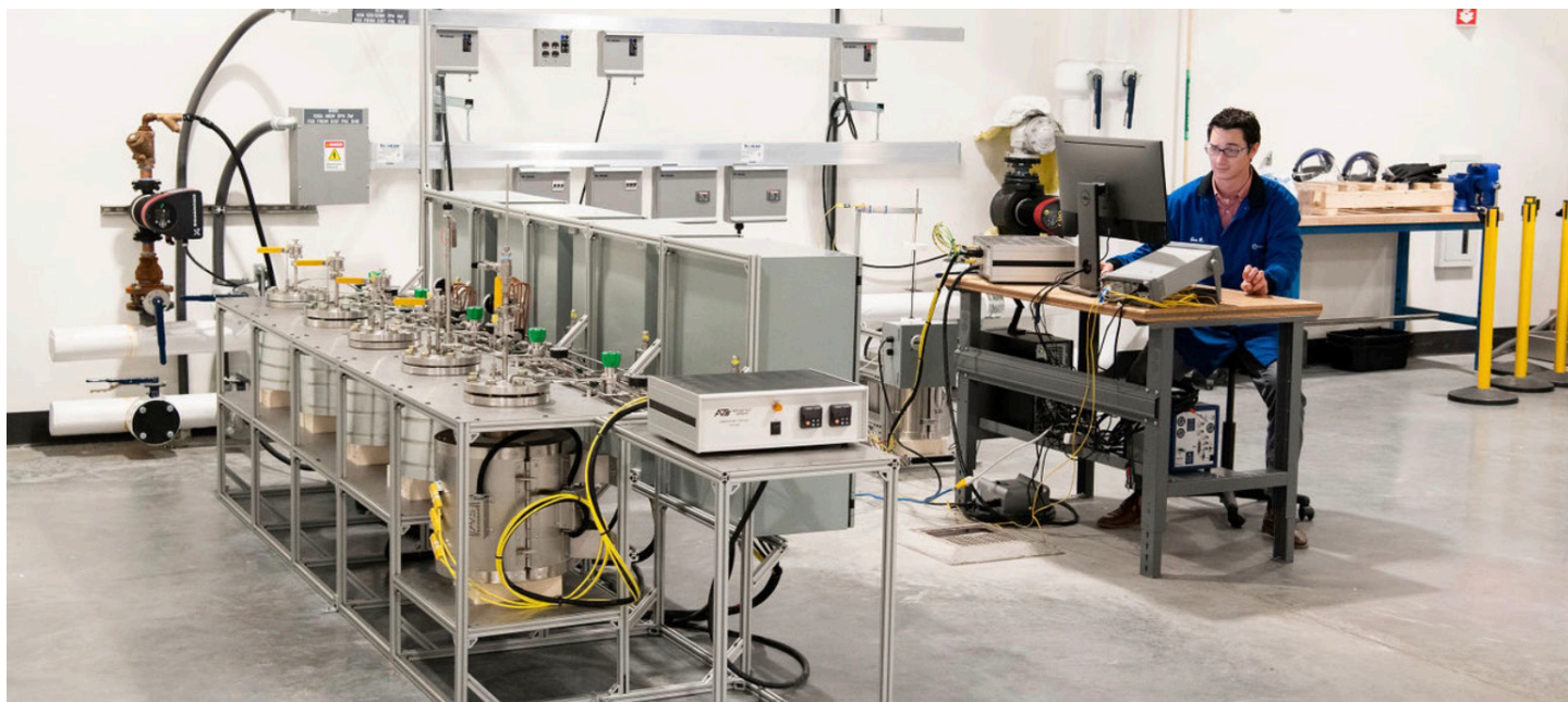
Gus Merwin, test engineer at Kairos Power, supervising a salt material compatibility test in the Kairos Power laboratory at corporate headquarters in Alameda, California.
