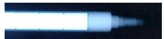
X-ray image of U_3Si_2 fuel segment
