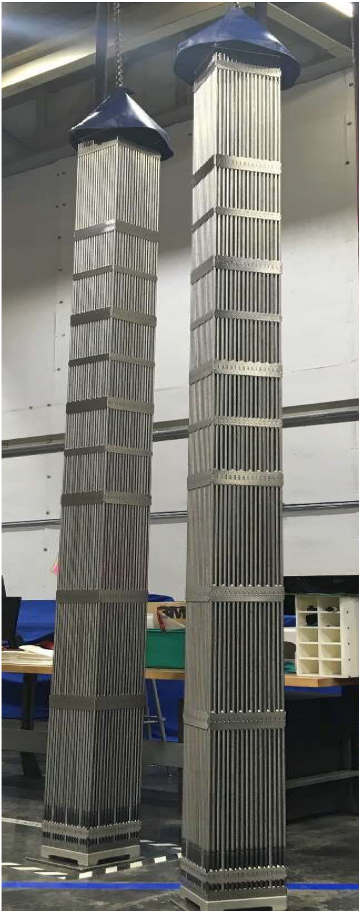
Two lead test fuel assemblies from Westinghouse-Exelon EnCore® Fuel Lead Test Rod (LTR) Program. The assemblies contained chromium-coated zirconium cladding for enhanced oxidation and corrosion resistance, higher density ADOPT™ pellets for improved fuel economics, and uranium silicide pellets. Photo courtesy of Westinghouse Electric Company, LLC.
