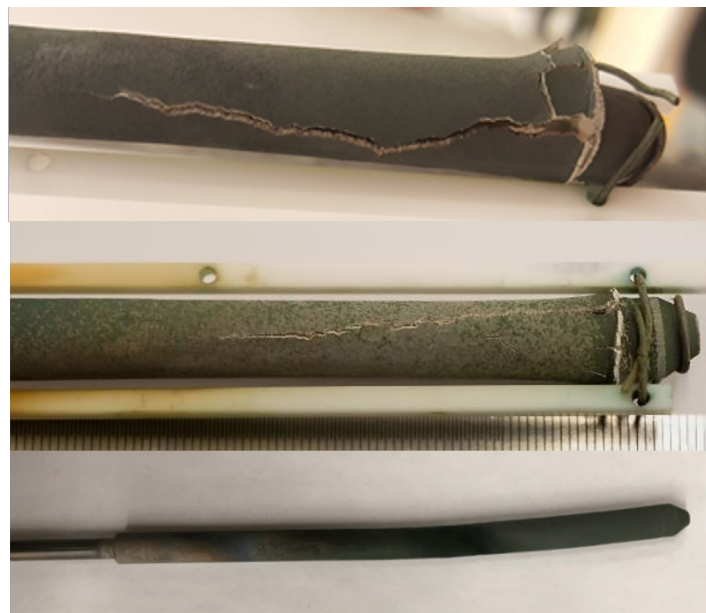
Exposure of three coated pressure tubes to 1200°C steam for 90 minutes and two new severe accident failure modes identified: Cr coating survived in all three tests, zipping due to presence of manufacturing coating defect took place in top two figures (top fresh, middle post-creep), ductile bending or buckling due to lack of thick oxide layer took place in bottom figure.
