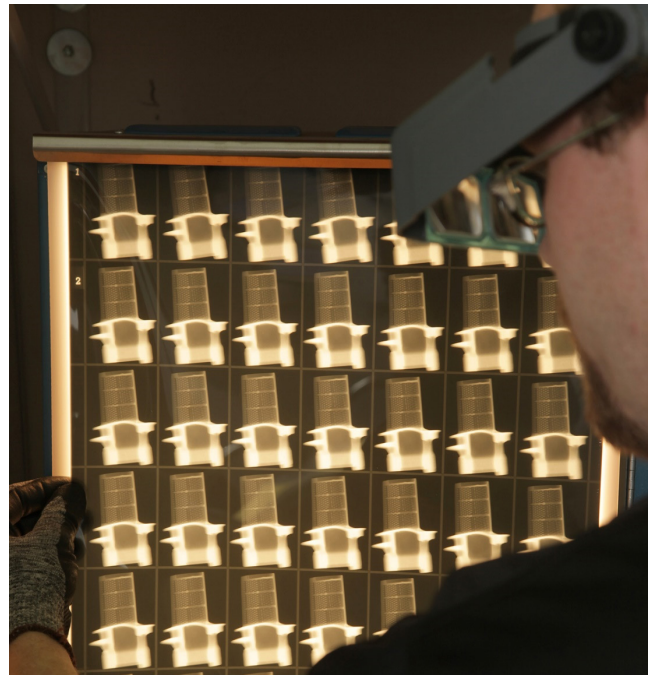
A neutron image of jet turbine airfoils acquired using the PULSTAR reactor’s Neutron Imaging Facility.
