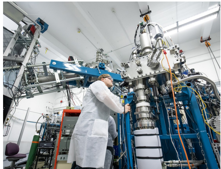
Multi-beam chamber for conducting dual and triple beam irradiations.
