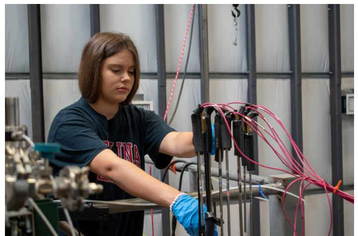
Shannon Henry, undergraduate research assistant, inserting interchangeable test rod at corner location. Possible test rods include simulated failed fuel rod, BWR water rod, PWR guide tube with dashpot, ordinary fuel rod (in this case with depleted uranium). Rods sticking out of the top of the chamber are the 12 heater rods.
