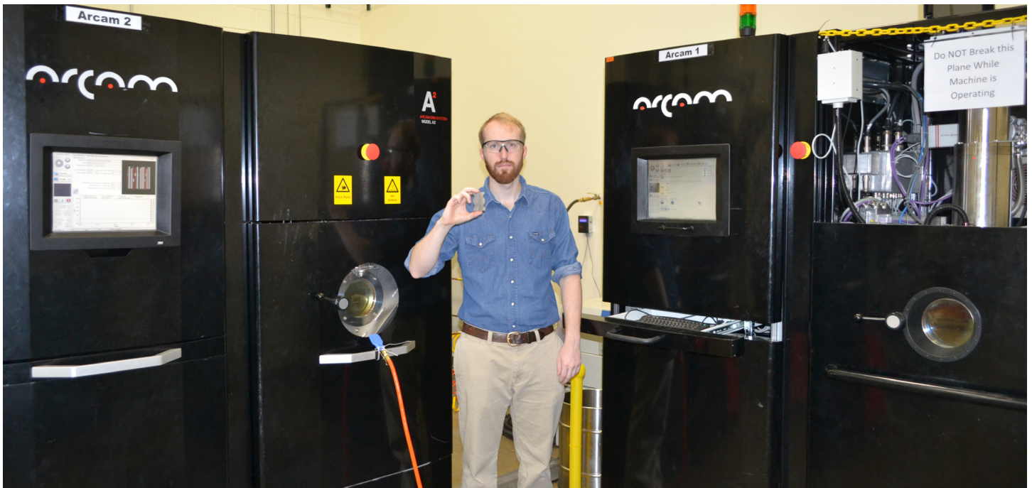
William Sames holding Inconel 718 fabricated by Arcam EBM® electron beam melting additive manufacturing, standing next to the machines at the ORNL MDF, where the DOE IUP-funded research was completed.
