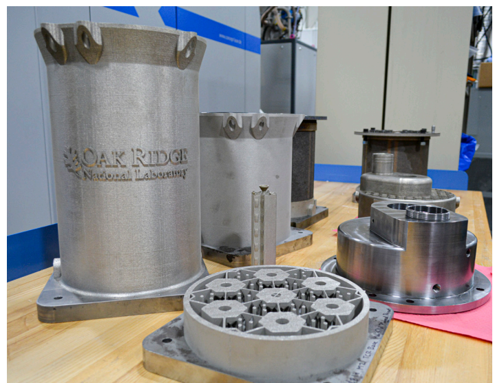
HTS IC's part is the shiny one, front right. This is a header for the TCR reactor vessel, which makes use of HTS IC's technology to embed sensors and thermal insulation, in addition to complex fluid passageways for reactor coolant. HTS IC's Metal Fusion Technology (MFT™) is a type of diffusion bonding additive manufacturing (DBAM) and was used to produce the component in coordination with the ORNL TCR team.
