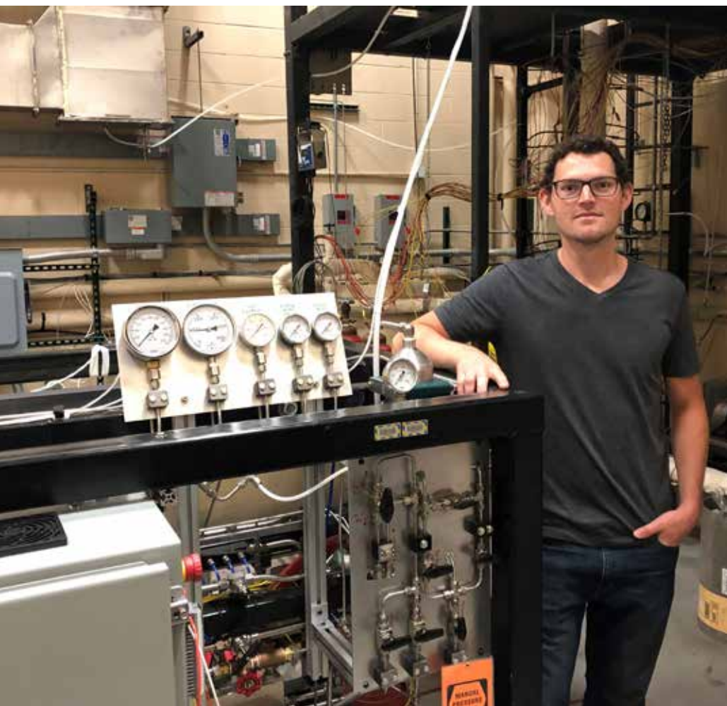
Graduate student Shaun Aakre standing next to a s\text{CO}_2 test rig connected to a molten salt loop getting ready to test a PCHE between salt and s\text{CO}_2 for the first time.
