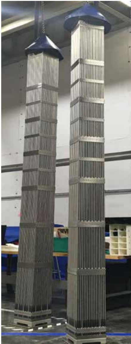
Two lead test fuel assemblies from Westinghouse-Exelon EnCore ® Fuel Lead Test Rod (LTR) Program. The assemblies contained chromium-coated zirconium cladding for enhanced oxidation and corrosion resistance, higher density ADOPT ™ pellets for improved fuel economics, and uranium silicide pellets. Photo courtesy of Westinghouse Electric Company, LLC.
