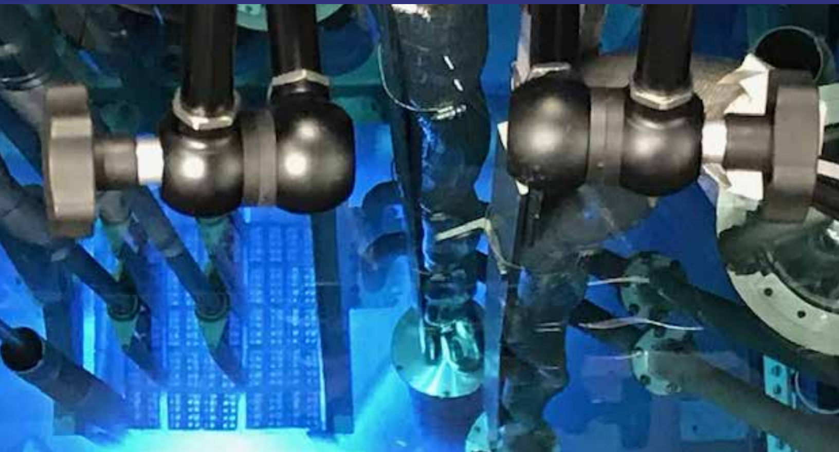
The conduct of irradiation tests in the PULSTAR reactor's pool in support of the Naval Reactor's program.
