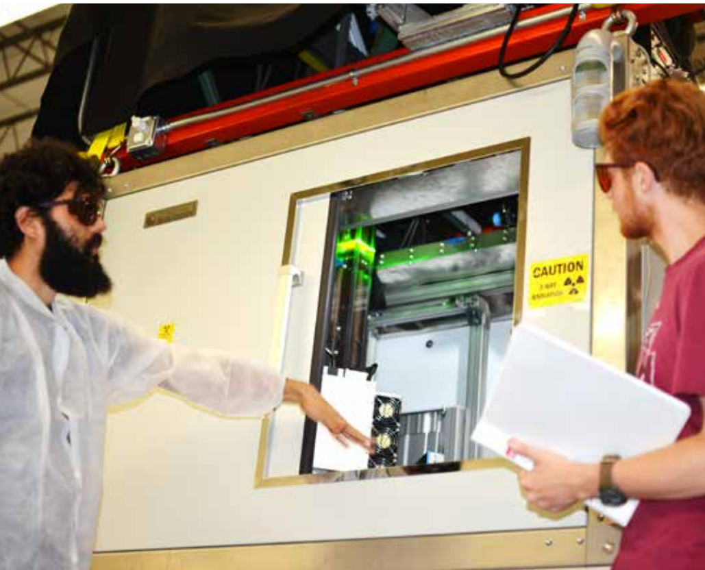
Students and the experimental system at the Thermal Hydraulic Research Lab (Texas A&M University). The system was awarded by NEUP Infrastructure for high-resolution multiscale measurements of single and multiphase flows featuring X-ray tomography, optical sensors and laser-diagnostics.
