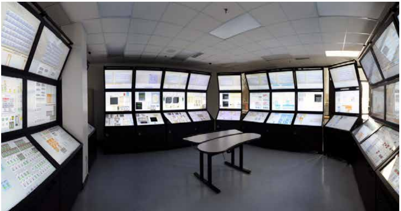
Operator support technology includes simulated diagnostic technology, an operator alarm display, and the fault scenario.
