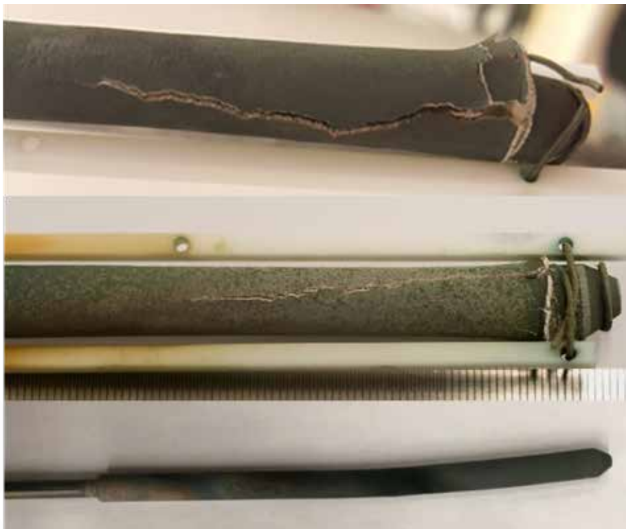
Exposure of three coated pressure tubes to 1200°C steam for 90 minutes and two new severe accident failure modes were identified: Cr coating survived in all three tests, zipping due to presence of manufacturing coating defect took place in top two figures (top fresh, middle post-creep), ductile bending or buckling due to lack of thick oxide layer took place in bottom figure.
