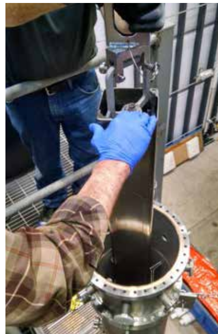
View of open test chamber showing installation of mock fuel assembly.
