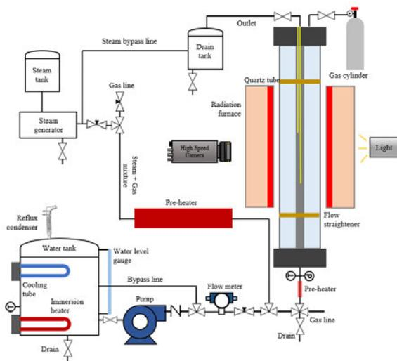
Fig. 1. Schematic design of single rod reflood facility
