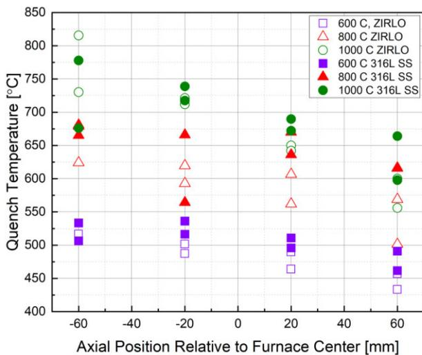
Fig. 3. Quench temperature vs axial position for 600, 800, and 1000 °C tests using 316L SS and ZIRLO.
