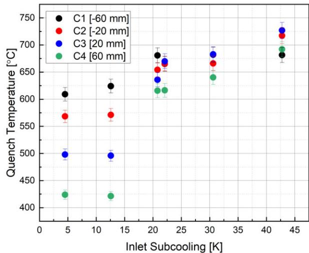
Fig. 4. Quench temperatures at various inlet subcooling for reflood tests with 800 °C initial temperature.
