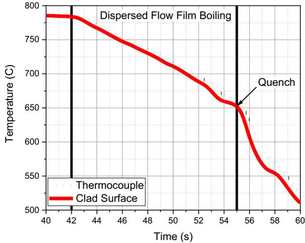
Fig. 2. Measured and calculated clad surface temperature during reflood of 316L SS cladding at 800 °C.
