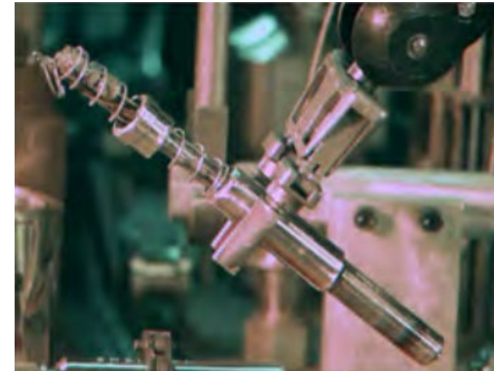
Disassembled fuel salt irradiation capsule with NaCl–UCl 3
