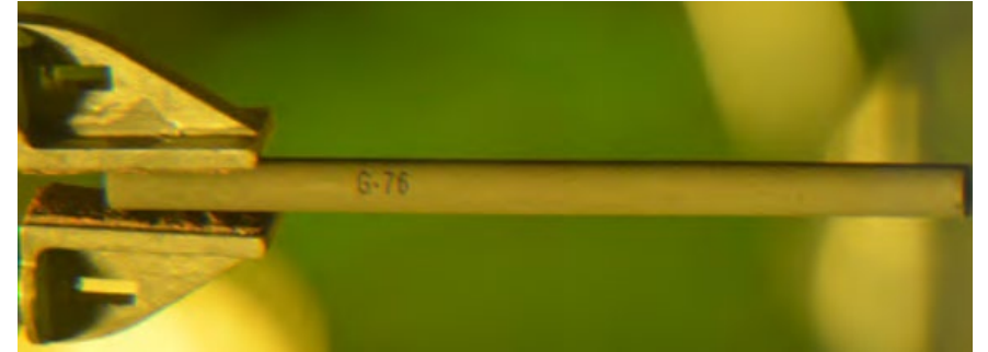
SiC clad pin after ATF-2 irradiation
