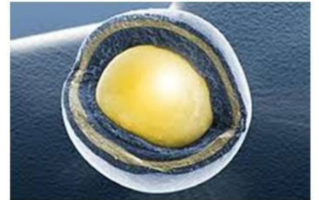
TRISO coated particle fuel
