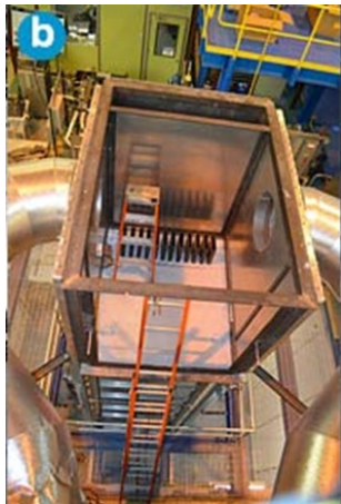
Natural convection Shutdown heat removal Test Facility (NSTF) for vessel cooling studies
