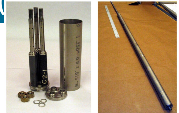
Figure A3. Photographs of a sample module during assembly and the fully assembled sample stack before insertion into the autoclave.
