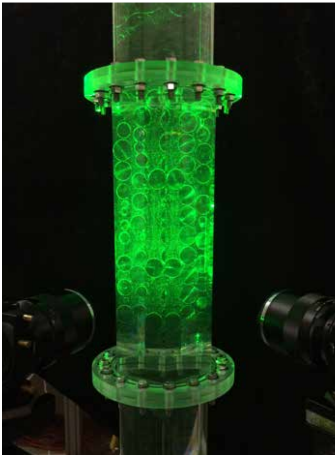
Texas A&M's advanced high-temperature reactor (AHTR) concept leverages a particle-based fuel format consisting of discrete spherical graphite pebbles arrayed in a packed bed architecture. Thermal regulation achieved via flow of gas (e.g., helium) or liquid (e.g., molten salt) coolants through the void spaces between pebbles in the bed (characteristic pebble diameters: ~ 6 cm, gas cooled; ~ 3 cm, liquid cooled).
