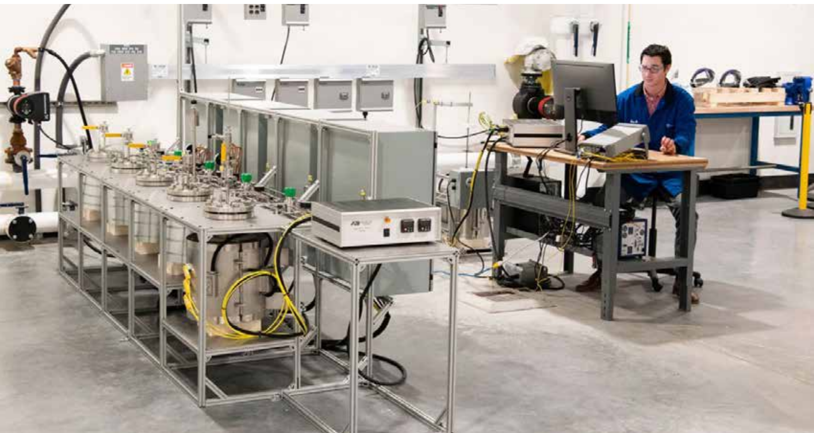
Gus Merwin, test engineer at Kairos Power, supervising a salt material compatibility test in the Kairos Power laboratory at corporate headquarters in Alameda, California.
